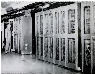
THE POOL ADDING MACHINES: The one at far left totals "win" bets, the center unit "place" bets, the one at right "show" bets.
